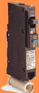
Arc Fault Circuit Interrupters (AFCIs) are new safety devices that replace standard circuit breakers in the electrical service panel. AFCI detect arc faults and shut down power to a circuit in milliseconds. Fire Marshall reports lists absence of AFCIs among the primary residential hazards associated with burns and fire-related injuries. These devices are so effective that the National Electrical Code requires that almost EVERY circuit in new homes be protected by AFCI's
